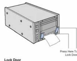
1. Unlock the paper exit door by pressing the open circles printed on the latches on either side of the door.
