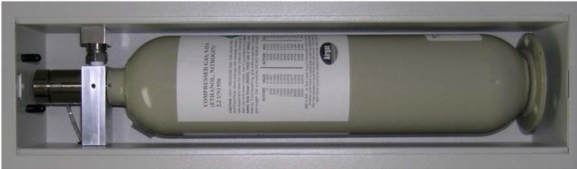
The dry gas standards are contained in a DOT approved, pressurized, dry gas tank that is connected to the EC/IR II through a single staged regulator. This tank contains a single-phased (gaseous), NIST traceable, mixture of nitrogen and ethanol that will produce a 0.082% at sea level. During a standard check performed by the instrument, the regulator and internal components within the EC/IR II will automatically sample and analyze the reference standard.
