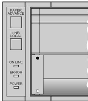
1. **PAPER ADVANCE button** – depressing advances paper out of the printer when it is “Off Line”. Press the “LINE/LOCAL” push-button until the “ON LINE” indicator goes off. Then, hold down the “PAPER ADVANCE” push-button until you have advanced the required amount of paper. Be sure to return the printer to the “On Line” mode before starting Subject Tests.
