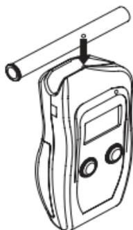
1. Take a new mouthpiece and insert it on top of the ALERT J5 device. With the display facing you, connect the mouthpiece to the device by aligning the holes and having the rimmed (larger) end of the mouthpiece pointing to the left.
