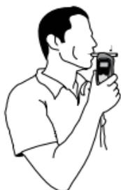
4. Take a deep breath and blow into the mouthpiece moderately, at a constant rate and pressure, until you hear a click sound (approximately 5 seconds). You should hear a continuous beep, indicating a proper breath flow. The click indicates the sampling process is complete.
